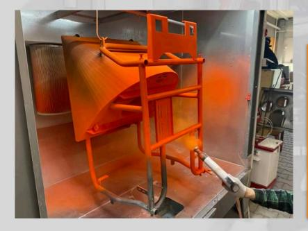
Powder coating is another very important stage of production. At this stage, the machine gains not only color and a nice appearance, but also excellent anti-corrosion protection. The paints we use are applied to the surfaces electrostatically and fired in a special chamber at a temperature of 200\*C, the process gives a 100% tight seal. paint coating.
